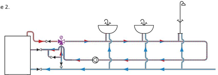
The ATM thermostatic mixing valve maintains the constant (set) temperature in the circulation circuit for several water taps and showers.
