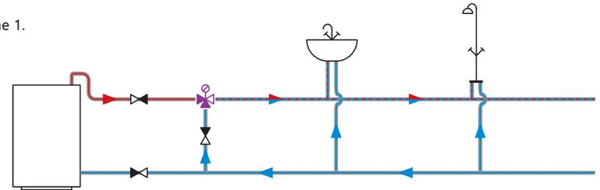
The ATM thermostatic mixing valve maintains the constant (set) hot water temperature in several water taps and showers.
