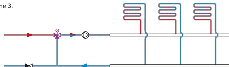
The ATM thermostatic mixing valve maintains the constant (set) temperature in the underfloor heating system.
