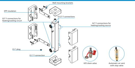
Vertical low loss header KSV 160 HW should be connected to the heating/cooling circuits according to the marking on the connections: red colour = supply, blue colour = return from the system/to heat or cold source.
