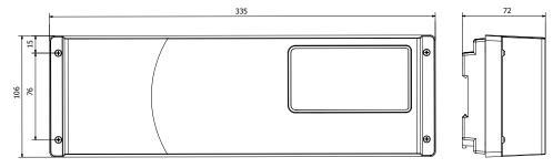
Figure 2. Dimensions of the FloorControl WB01 D-8-24 wiring box
