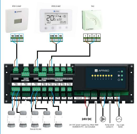
Figure 4. Electrical connections
