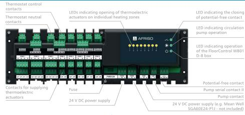
Figure 1. Structure description of the FloorControl WB01 D-8-24 wiring box
