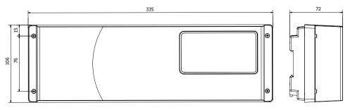
Figure 2. Dimensions of the FloorControl WB01 D-8-230 wiring box
