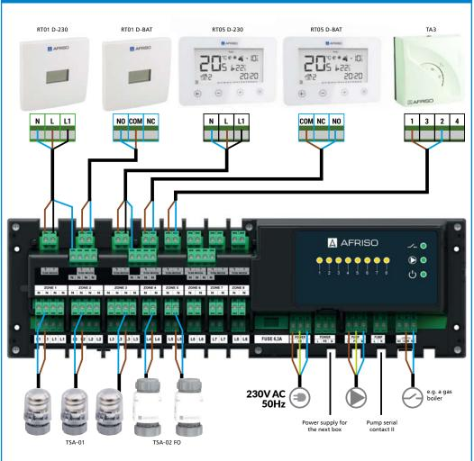
Figure 4. Electrical connections
