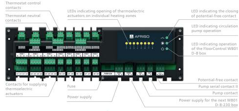
Figure 1. Structure description of the FloorControl WB01 D-8-230 wiring box
