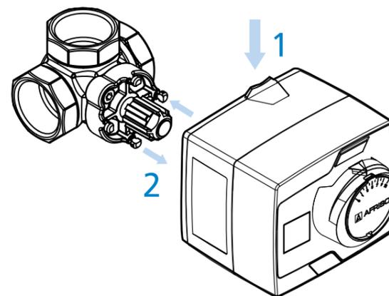
Fig. 2. Mounting/dismounting of an ACT ProClick controller on a valve
