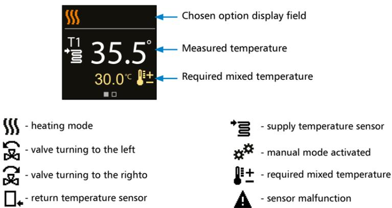
Fig. 10. Description of the symbols displayed on the controller.
