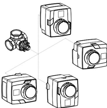
Fig. 3. Possible mounting positions
