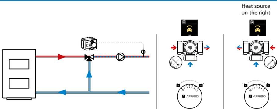
Fig. 6. Diagram with the mixing valve mounted on the supply pipe to maintain a constant temperature of the medium in the system.
