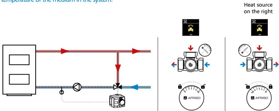
Fig. 7. Diagram with the mixing valve mounted on the return to the heat source, in order to protect the heat source against low-temperature corrosion.
