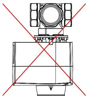
Fig. 4. Improper mounting position
