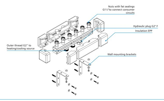
Boiler manifold KSV 125 - 160 kW should be connected to heating/cooling circuits accordingly to the markings on the connections: red colour = supply, blue colour = return from the system/to heat or cool source. Consumer circuits should be connected via flat sealings. However, sealings or suitable sealant, e.g. Teflon tape should be used to seal the connections of the heat/cool source circuit.
