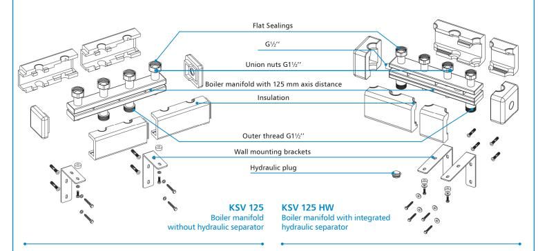
Boiler manifolds KSV 125 are used for distribution of heating water in sealed heating systems. Heating circuits should be connected via flat sealing union nut G1½". The same sealing should be used to connect the product with the boiler circuit.
