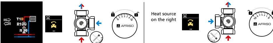
Fig. 10. Diagram with a 3-way mixing valve mounted on the supply pipe (radiator or manifold heating). This version allows for connecting more controllers using BUS communication.
