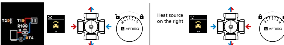
Fig. 11. Diagram with a 4-way mixing valve (radiator or manifold heating) with the return temperature protection function active.
