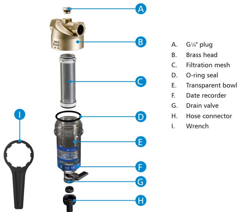
Fig. 2 Construction of the AWF water filter
