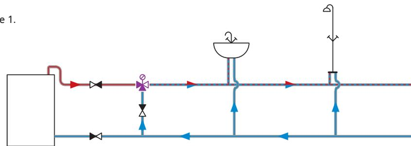
The ATM thermostatic mixing valve maintains the constant (set) hot water temperature in several water taps and showers.
