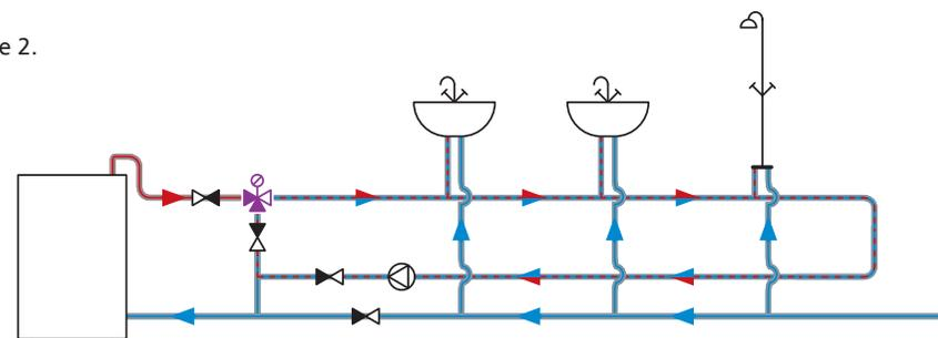
The ATM thermostatic mixing valve maintains the constant (set) temperature in the circulation circuit for several water taps and showers.
