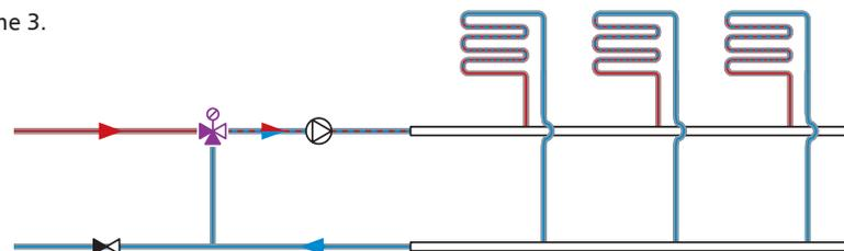
The ATM thermostatic mixing valve maintains the constant (set) temperature in the underfloor heating system.
